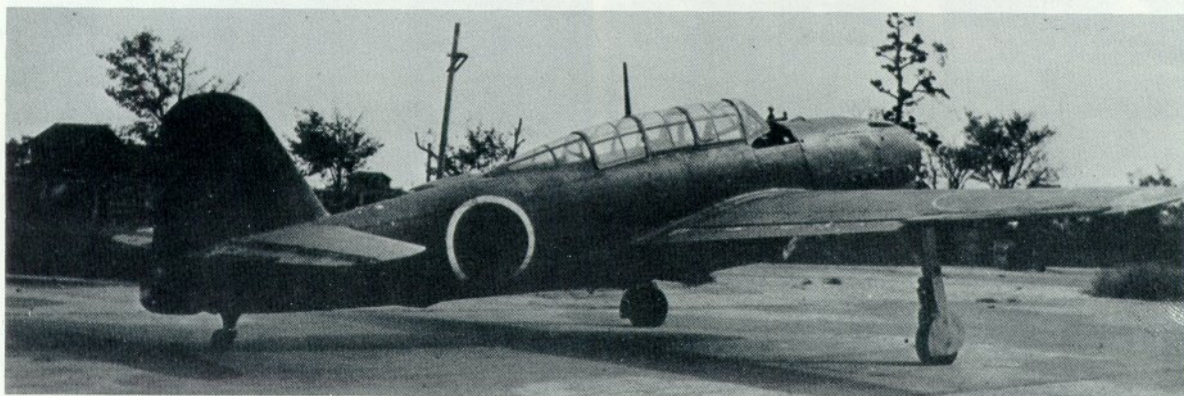
Following the cease fire at the end of the Pacific War in August 1945, the majority of Japanese combat aircraft – like this D4Y2 – were demobilized by the simple expedient of removing propellers.
