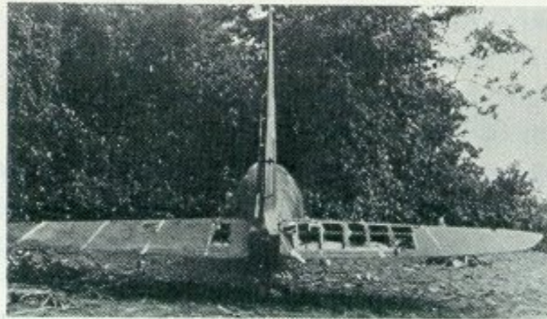
A damaged tail section of a D3A1 the white stripes on the tailplane are angles of fire for the rear gunner.
