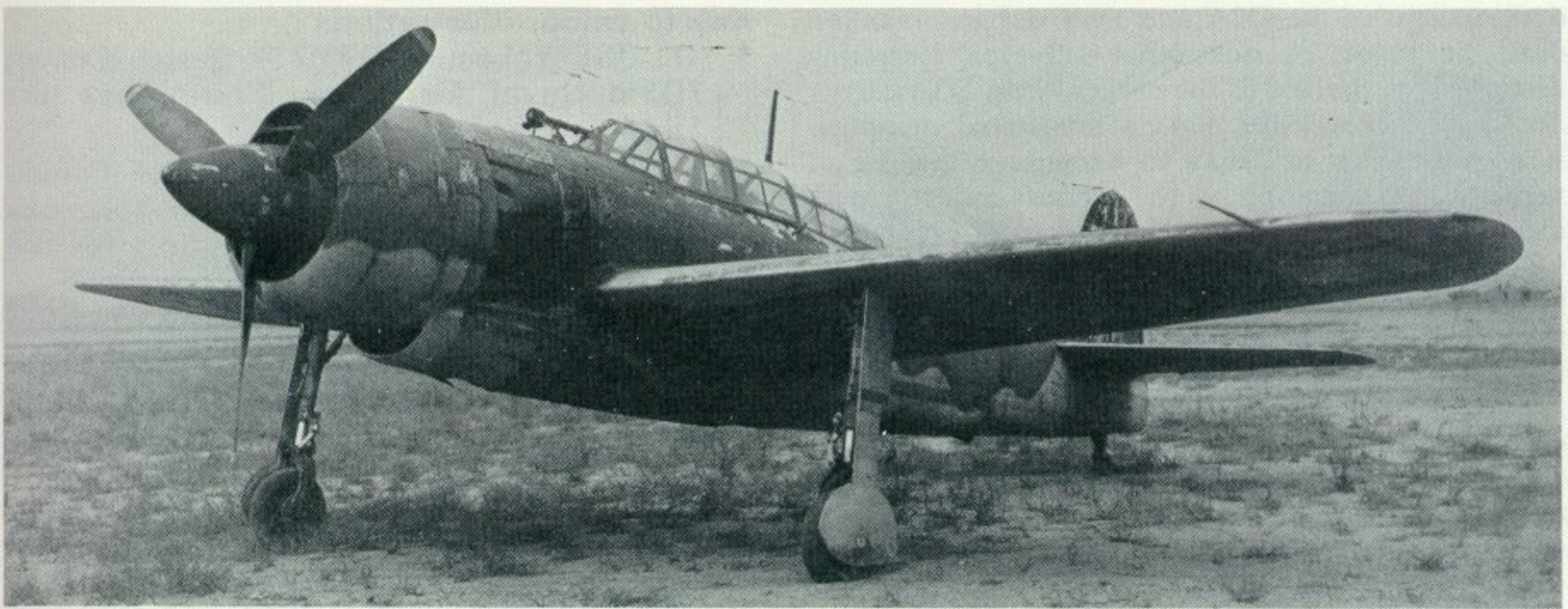
A D4Y3 of the 601st Naval Air Corps, this exceptionally clear view shows to good effect the bulky radial which was installed on the slim fuselage of the Suisei .
