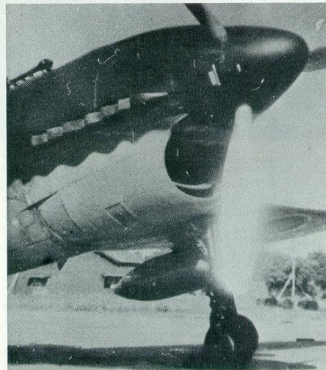
A D4Y2 in close-up shows to advantage the pilot's external gun sight and one of the two 330-litre under-wing drop tanks. (Photo: via Major Robert C. Mikesh)
