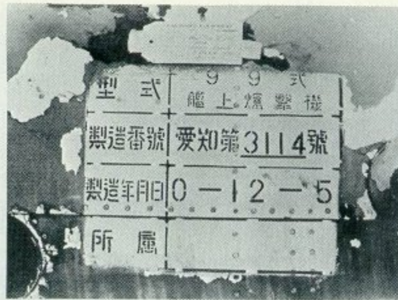
The manufacturer's identity panel from a D3A1 shot down at Deba, Papua, New Guinea on September 3, 1942. Reads: top line, Type 99 Carrier Bomber; second line, serial number 3114; third line, date of manufacture, December 5, 1940.
