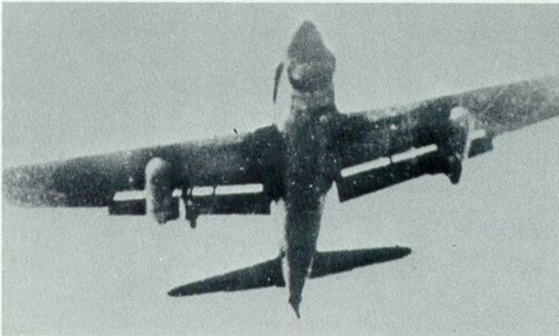
A D4Y1 in flight with under-wing drop tanks fitted. The slotted flaps are shown to advantage. (Photo: Real Photographs via Dr. R. J. Francillon)
