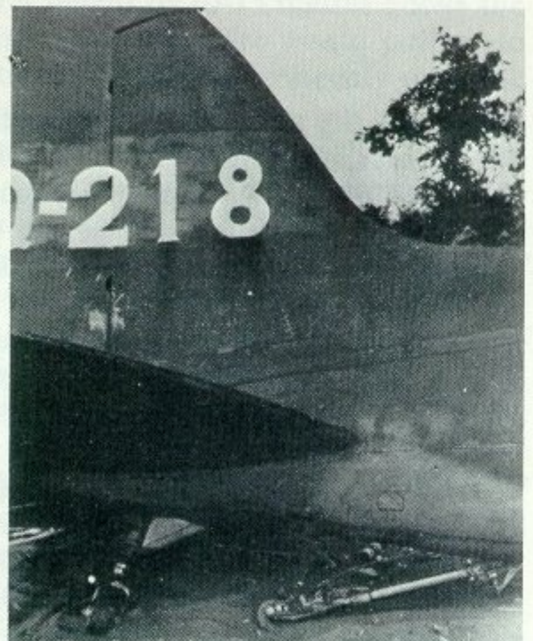
A close up of the tail-wheel and deck arrester hook of a D3A1 of the 2nd Naval Air Corps. (All photos: via Major Robert C. Mikesch)
