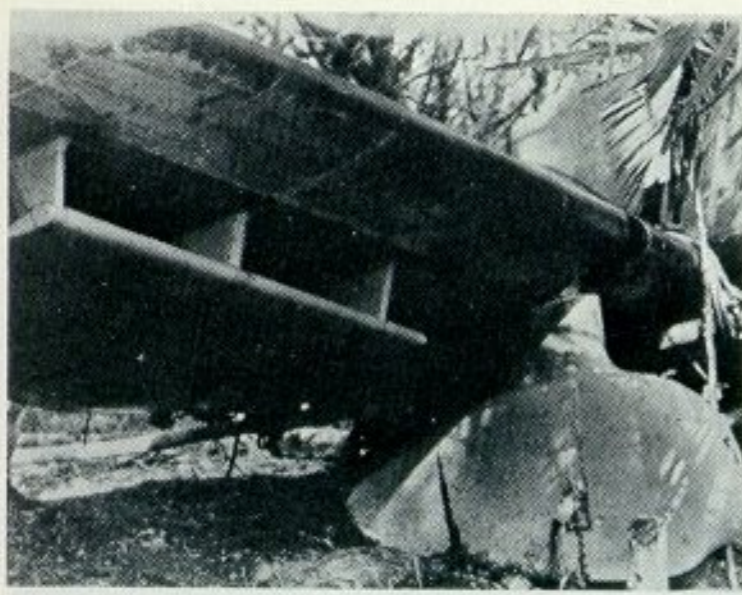
A close-up of the fixed undercarriage and dive-brake of the D3A1 carrier bomber.
